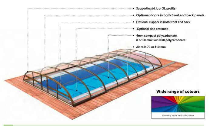
The enclosure is delivered with rails on the left and right side in the length of the enclosure. For moving the enclosure outside of the area of the pool, we recommend buying extension rails. More information on enclosure equipment, colour options and technical details can be found on pages 98 - 105.
