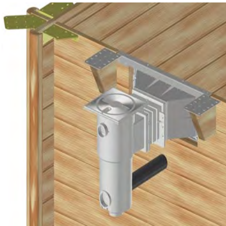
Figure 23 – Mounting the skimmer bracket
