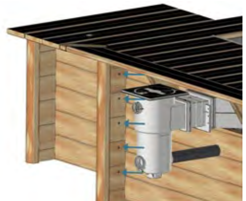
Figure 63 – Fastening the cover pit to the pool
